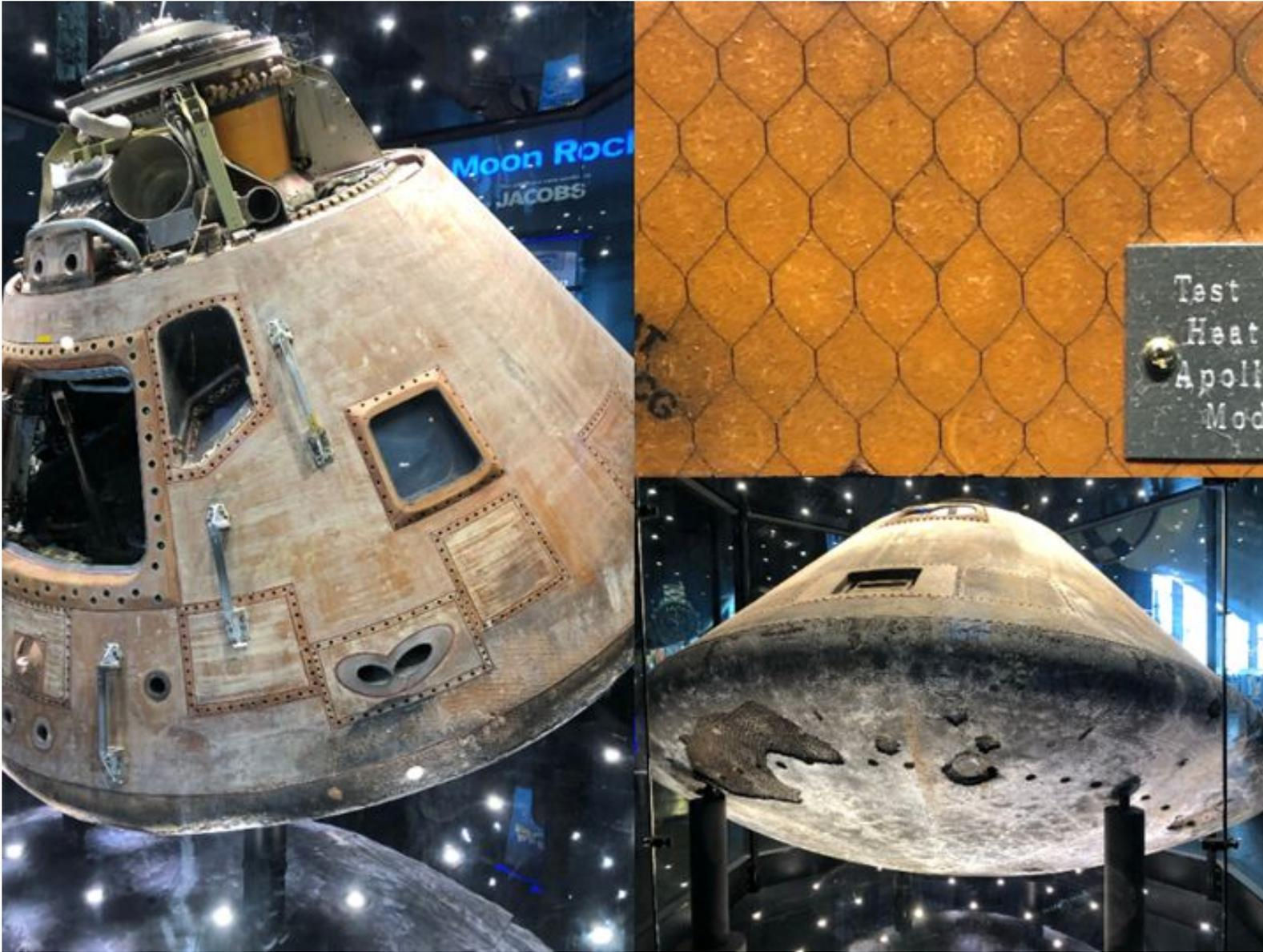
*Apollo's* heat shield made of epoxy phenolic novolac resin in a fiberglass honeycomb
