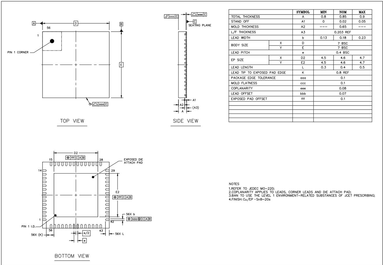
Figure 8: QFN56 (7x7 mm) Package, for ESP32-S2FN4R2
