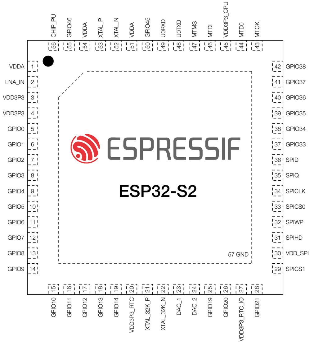
Figure 3: ESP32-S2 Pin Layout (Top View)
