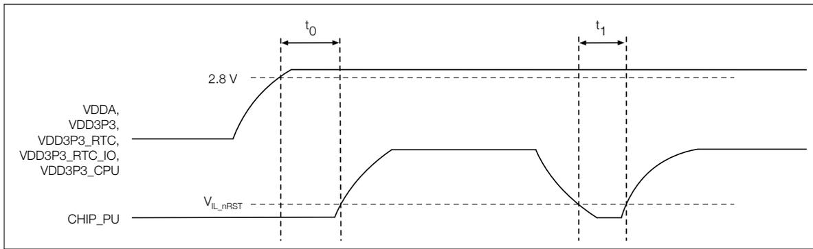
Figure 5: ESP32-S2 Power-up and Reset Timing
